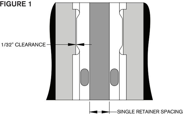
**STEP 5:** Install the two single retainers back-to-back in the gap between the last two pads. (See Figure 1) Use the same welding procedures and clearances as described for the double retainers. The space between the single retainers will vary slightly according to the actual pulley diameter. However, the gap should not exceed the limits given in Section 1. Otherwise, non-standard installation is required.
